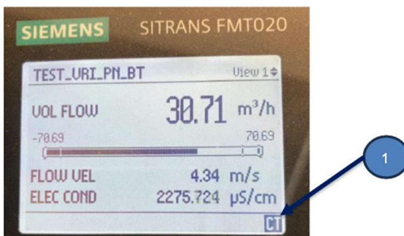
Picture 4 - Identification of CT mode enabled on FMT020 HMI
