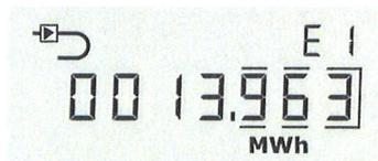
If the meter is set to be an inlet meter, the "Inlet arrow" is displayed.
