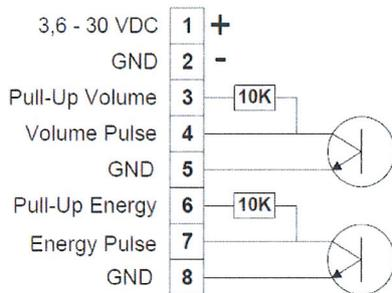
When Pulse Interface type 66-99-143 is connected to power supply or battery, the unit is placed on the meter, and the meter is in test mode, the following pulses are transmitted:
