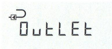
If the meter is set to be an outlet meter, the "Outlet arrow" is displayed.
