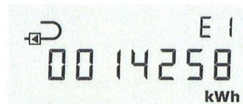
If the meter is set to be an outlet meter, the "Outlet arrow" is displayed.
